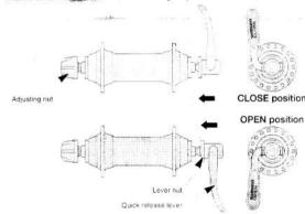
The clamping strength is adjusted by turning the adjusting nut. When the nut is turned in a clockwise direction, the clamping strength increases, and when the nut is turned in a counterclockwise direction, the clamping strength decreases.
